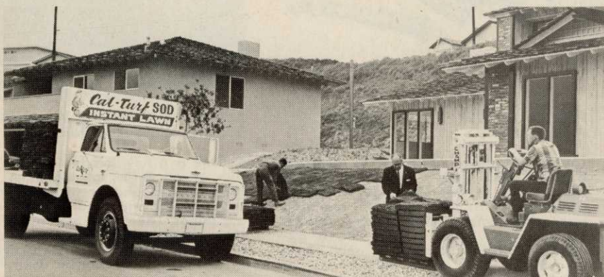
Champ fork lifts load trucks at the field, are towed to delivery site, then unload and move sod to point of laying.
