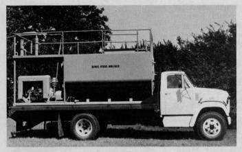
Bowie Industries, Inc., Bowie, Texas, introduces the Bowie Imperial 2500 Hydromulcher, featuring a 2,500-gal. capacity extrathorough agitation and central controlled spraying tower. The unit is designed for fast, simultaneous application of seed or sprigs, fertilizer wood fibre and water on steep slope, roadway, public works, reforestation, golf course, park, home lawn, and housing project terrains. It is equipped with the patented Bowie pump. For more details, circle (702) on reply card.
