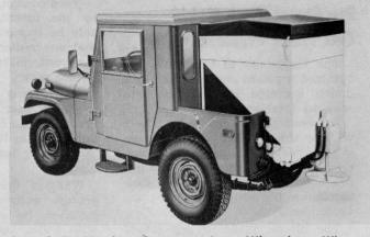
Central Engineering Company, Inc., Milwaukee, Wis., announces a new AUTO-SPREADER, Model A-100. Unit is a selfpowered, self-contained, portable chemical and material spreader, holding one cubic yard of material. It can be easily mounted in the cargo area of a small service vehicle, or attached to a tractor three-point hitch. It is equipped with an instant on-off control switch for spot spreading of paved and turfed surfaces. For more details, circle (703) on reply card.
