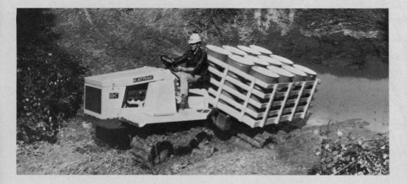
Katrak Vehicle Co., Canby, Ore., claims its revolutionary 4-track drive Katrak K-60 hauls heavy I o a ds through knee-deep swampy or sandy areas with ease. Carries payloads of up to 2½ tons and travels at speeds to 25 mph. Powered by 302-cubicinch, 200 hp Ford industrial engine. Turning radius is 11 feet. Eight speeds forward, two reverse. For more details, circle (702) on reply card.
