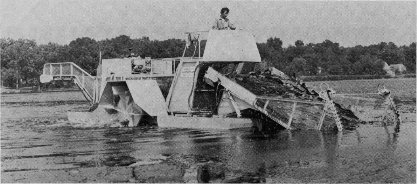
The basic member of Aquamarine's Aqua-Trio is the H-650 Harvester. It cuts a swath eight feet wide and five feet deep. Live bed hold packs weeds automatically, unloads automatically.
