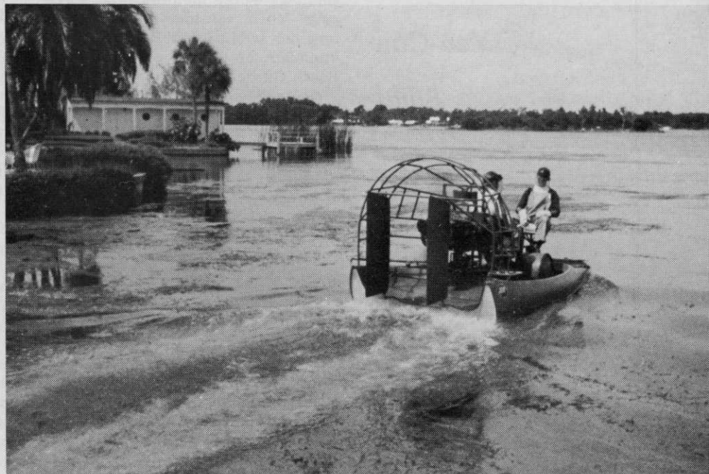
Hurricane Fibreglass "Aircat" has proved the ideal vehicle for aquatic weed treatment, floating over the surface without picking up weed particles. Normal operation is to introduce chemicals below the surface as shown here. The airboat is equipped with an F. E. Myers 10 gpm pump.
