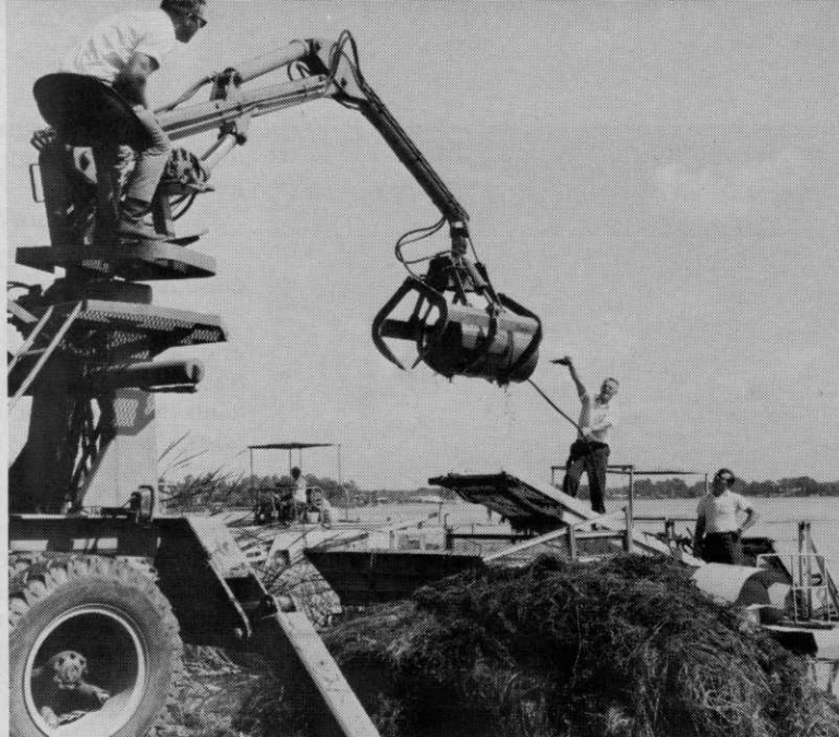
Roy Campbell shows how a Prentice grapple hook loader, ordinarily used for handling logs, comes in handy during aquatic weed harvesting. He's refueling a harvester.
