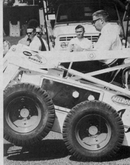
Bobcat by rearing it backward and pivoting it to the opposite direction. It was equipped with a front scoop.
