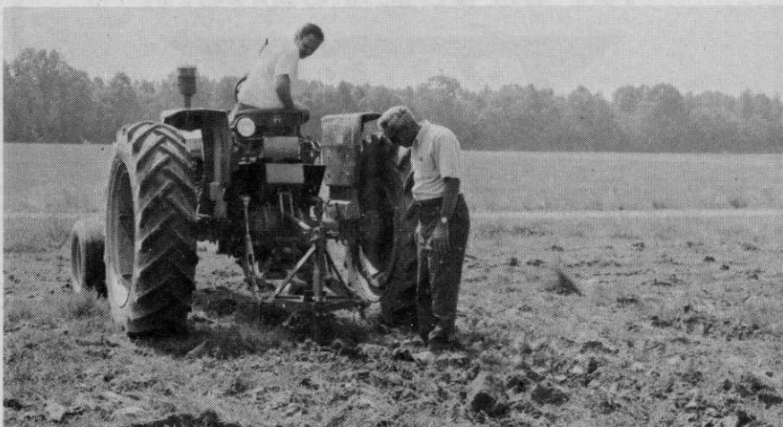
A sub-soiler is used to counteract compaction of heavy equipment.
