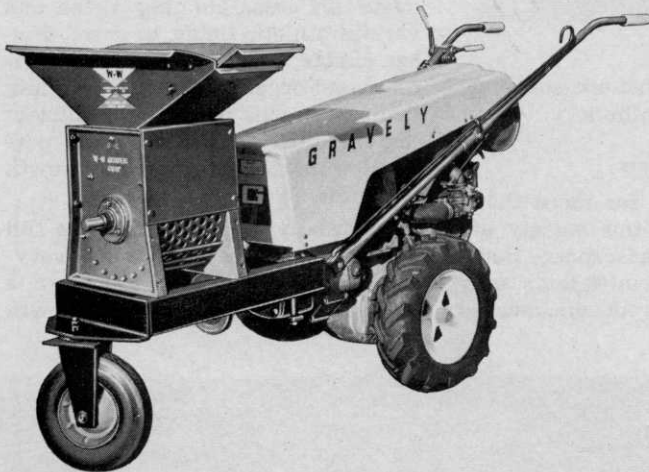
W-W Grinder Corporation offers a shredder that can be powered by a garden tractor with the use of a V-belt pulley. A stabilizer bar is provided which is simply and easily attached to most garden tractors. This Model 5 unit provides up to six yards per hour capacity.
