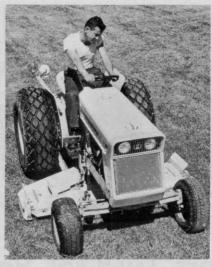
International Harvester Company, Chicago, has added four new pieces of equipment to broaden the application of its 15 hp. International Cub 154 Lo-Boy. The company has added the 3142 42-in. (left) and the 3160 60-in. rotary cutters to cut tall grasses where debris may be encountered. The other attachments are a rototiller with a 42" cut and a snow thrower with 24" auger and 180° swivel discharge chute to clean up to a 54" swath. For more details, circle (703) on reply card.
