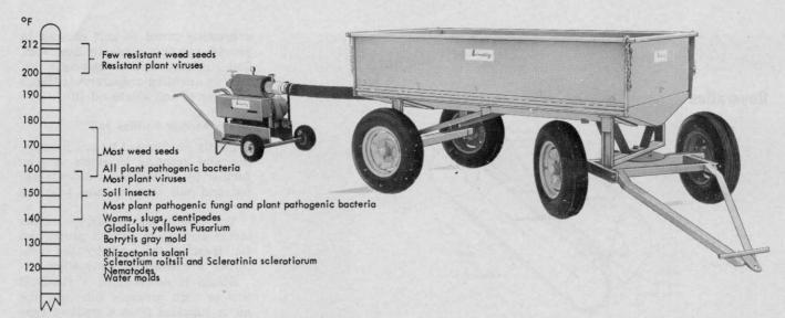
Lindig Mfg. also offers a steam aerator and a soil cart. The aerator provides low-temperature steam sterilization that does not harm beneficial soil pathogens. Steam is injected into the soil cart at a temperature range between 145 and 165 degrees for a period of 30 minutes. As the chart indicates, most plant-damaging micro-organisms, insects, viruses and weeds can be destroyed. The aerator and cart come in two sizes.
