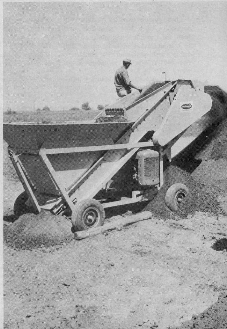
The Royer Paul Bunyan 360T is what its name implies, the biggest of the Royer line with a capacity of 100 cubic yards per hour. Its receiving hopper will handle buckets up to two cubic yards. It can be towed at highway truck speeds.
