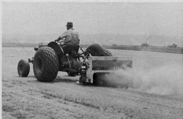
To minimize compaction, Latta and Scholes have mounted field equipment on airplane tires . . .
