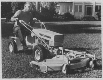
Gravely Corp., Clemmons, N. C., now offers a riding-walking Convertible tractor in 7.6, 10 or 12 horsepower. Features include all-gear drive, instant forward and reverse, rear engine
