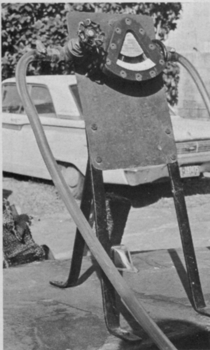
This flow meter, which shows how much herbicide is entering the water, is in the operator's constant view at the front of the airboat.
