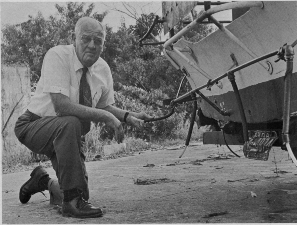
Florida's Charlie Johnson shows his airboat's flexible, plastic downspouts through which acrolien is released into lakes and canals. Spouts are wrapped in springs to keep them pointed downward.
