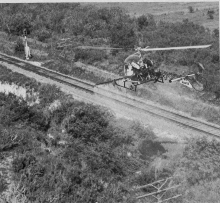
Invert emulsion enables ROWCO pilots to target herbicides on water or right-of-way from up to 75 feet in the air and still control pesticide drift.
