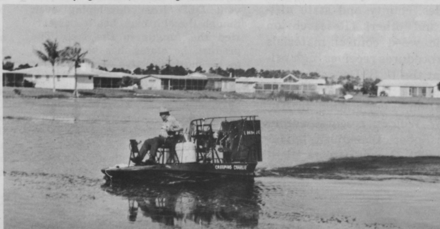
"Creeping Charlie," releasing herbicide underwater, skims over lake's surface.
