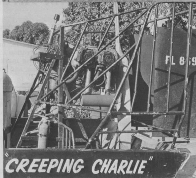
"Creeping Charlie," releasing herbicide underwater, skims over lake's surface.
