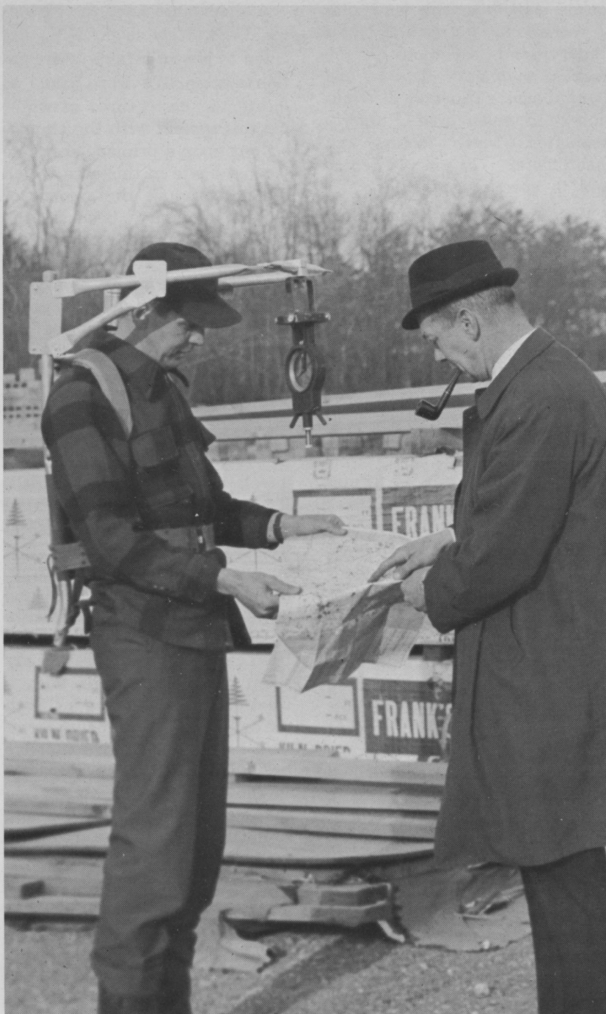
Aquatometer being used to locate water supply at new school site. Transporting instrument is Dick Jamieson and checking plot map is George (Hap) Jamieson, both experienced men in using the water magnetometer.
