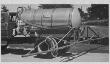
Clark's truck-mounted sprayer has 1000-gal., stainless steel tank with rubber-lined saddle. Full-length sparging tube is welded to tank bottom for agitation. Model U-37, 10-row channel boom shown has 1" hose, resists corrosion. Choice of engine and pump units. Shown is 7 H.P. Wisconsin engine with M.P. (flomax 10) 180 GPM centrifugal pump. Accommodates most fertilizer solutions, mixed, liquid and suspension materials, says Clark's. For more details circle (706) on reply card.
