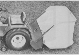
Fort Myers Iron Works, Fort Myers, Fla., makes available Litter-Whisk attachment for Wheel Horse tractors. Unit is 37" wide, whisks up 15 bushels of cuttings, leaves (even wet ones), pine needles, paper, etc. Tractor-mounted, it simplifies dumping and maneuverability. Hopper can be emptied from driver's seat. For more details circle (709) on reply
