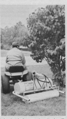
Lakes Supply Company, Inc., Dundee, Ill., introduces a turf weed control unit, available in three models, to curb the "drift" of spray weedicides that kill plant life. Called "The Drip," it operates by dripping liquid weed killer onto a roller, coating it with a film. The damp roller kills the weeds it contacts. Model 101, illustrated, is equipped with a 36" wide roller and a 151/3-gal. capacity tank. For more details, circle (706) on reply card.
