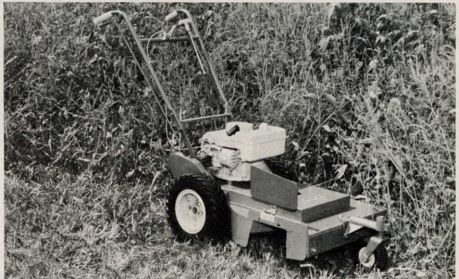
Bunton Co., Inc., Louisville, Ky., is marketing its "Super Twenty-one"—a heavy-duty, self-propelled rotary power mower with 4 HP engine and 2-qt. fuel tank. Designed for extra traction and "mowability" in rough areas and on grades, Bunton's new unit offers adjustable cutting heights from 2 1/2" to 5 1/2". Features include finger-tip guiding, blade control on handles, trimming with either side, adjustable front guard, fold-down handles and belt and chain guards. Smaller model also available. For more details circle (706) on reply card.
