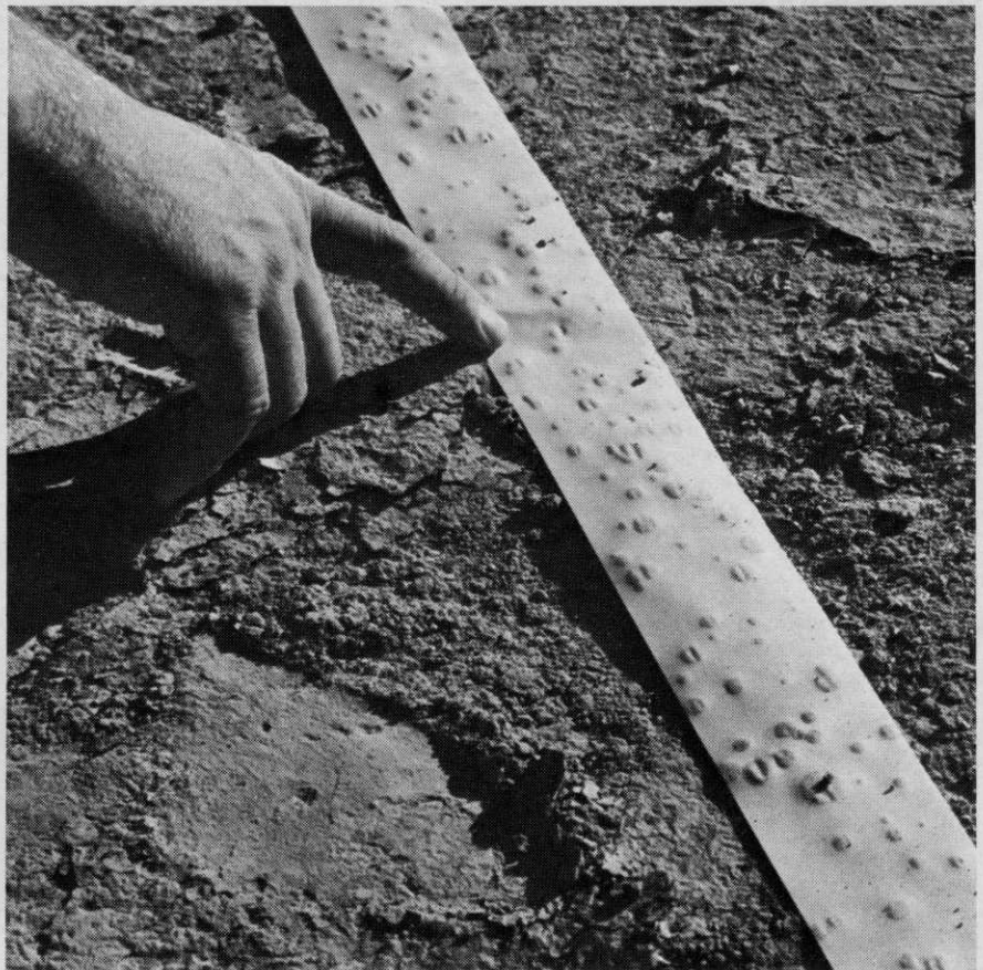
Spray droplet pattern from microfoil delivers series of droplets which are nearly uniform in size.
