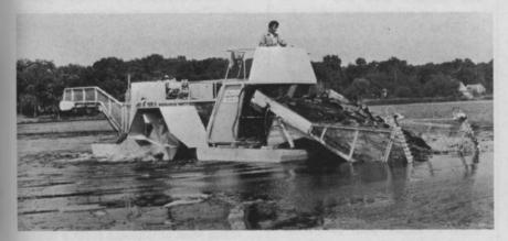
A complete mechanical water weed removal system is offered by the Aquamarine Corporation of Waukesha, Wis. The key unit of the Aqua-Trio, as the system is called, is the H-650 harvester shown above. The other two units are a weed transporter and a shore conveyor. Weeds are cut, transported to shore, and loaded into trucks without being handled manually. The harvester cuts an 8-ft. wide swath to a depth of 5 ft. For details, circle (711) on reply card.
