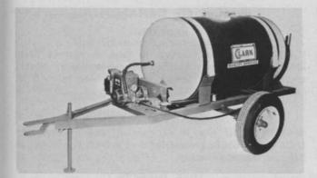
Clark Mfg. Co., Atherton, Mo., introduces a two-wheel Model "GL" trailer sprayer. The 200-gal. fiberglass tank will handle engine-driven roller pumps for low-pressure spraying, or engine-driven piston pumps for high-pressure spraying. The unit comes with trailer,  $6" \times 14"$  wheels (less tires), 50-ft. handgun hose, hose reel, 5 HP engine and choice of pumps, saddle, straps, hose and fittings. It's adaptable for spraying with a boomjet nozzle. For more details, circle (707) on reply card.
