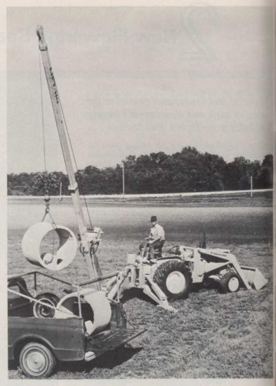
Allis-Chalmers, Topeka, Kan., adds its new Model 631 crane boom for use with its 1-600 loader-backhoe industrial tractor. The telescoping boom mounts on the backhoe in place of the bucket and dipper arm. It has a 2000-lb. maximum lifting capacity at a 12-ft. radius from the backhoe center point. When fully extended, the three-position boom has a 31-ft. maximum reach; a 25-ft. mid-point reach and a 19-ft. fully retracted reach. For more details, circle (702) on reply card.
