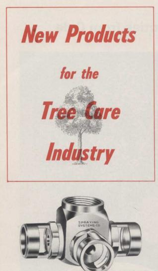
Spraying Systems Co., Bellwood, Ill., introduces largecapacity No. 12381SS-SC jet agitators to provide turbulence to keep wettable powders in uniform suspension. As liquid streams from agitator outlets, surrounding liquid is drawn through open side ports of the siphon caps, causing agitation. The brass or stainless steel units, in four capacities, feature a ¾" NPT female inlet connection. For more details, circle (701) on reply card.
