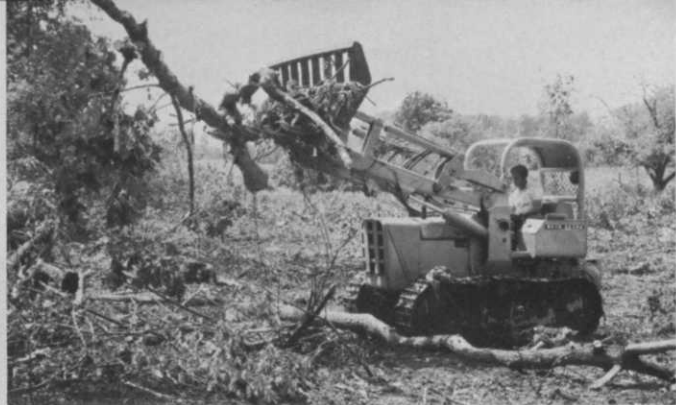
A lift rake and brush chipper enable Jaflo to clear fast and clean with minimum damage to other landscaping.
