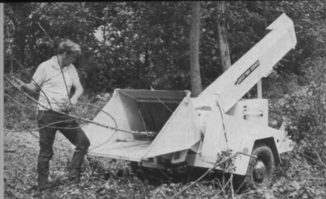
A lift rake and brush chipper enable Jaflo to clear fast and clean with minimum damage to other landscaping.
