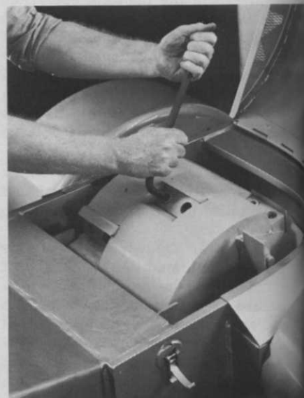
Staggered knives cut smoothly, shave material uniformly on this cylinder-type chipper, a Mitts & Merrill. Knives are double-edged and are easily accessible for reversing and sharpening.
