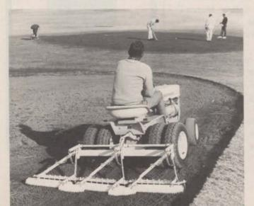
International Harvester Company has recently developed its new Sand Trap Rake in conjunction with the needs of a greenskeeper at one of the nation's leading golf courses. This new unit, International Harvester contends, cuts manhours required for raking sand traps by 50 per cent, which frees maintenance workers for other chores. Uniform penetration of the rake eliminates hardpan and cultivates weeds and grass out of traps, according to the company, For more details circle (703) on reply card.
