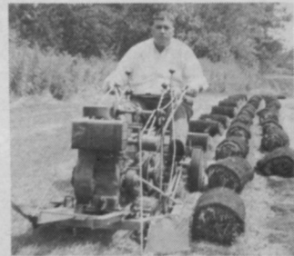
Sod roller was designed and built by Don Morrill for use on Shamrock Turf farm. Unit as yet is not commercially available.
