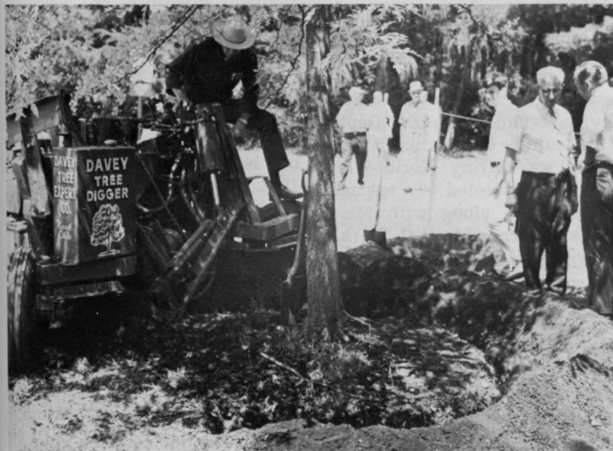
Davey Tree Expert Co., Kent, O., exhibited the new Davey tree digger. Machine trenches circle completely around tree for standard moving process.
