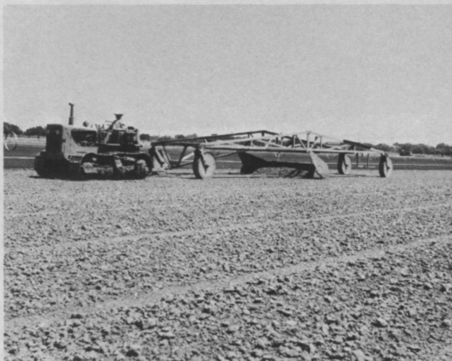
Land leveler is used to float soil base, knocking off the high spots and filling low areas for level seed-bed.
