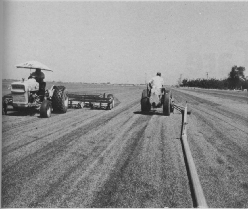
Tony Mello, left, and John Nunes demonstrate two manpower saving features of Nunes operation. Mower, of standard carrier design is equipped with 17-foot cut to eliminate mowing time, and to relieve compaction. Pipe mover efficiently shifts pipe ahead of mower.
