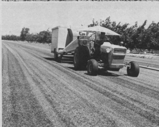
Special vacuum sweeper developed by Nunes is equipped with flotation wheels and own power plant for hydraulic and vacuum.
