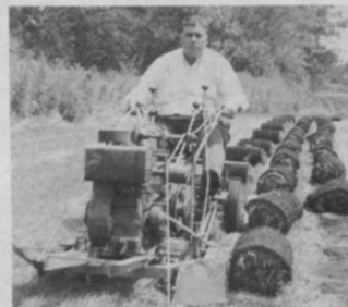
Sod roller was designed and built by Don Morrill for use on Shamrock Turf farm. Unit as yet is not commercially available.
