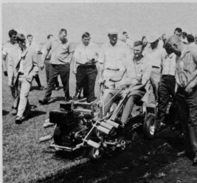
Newest piece of sod equipment on display was Ryan sulky, roller attachment for standard Ryan cutter.
