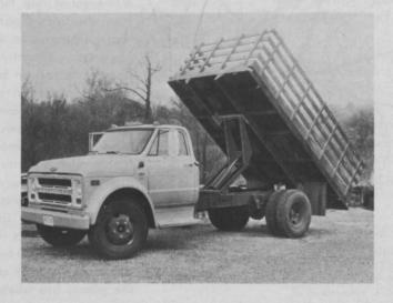
A new TH model series of Goebel Scissors Hoists can be installed on any straight truck with a 1 to 2½-ton chassis. Goebel's dashboard - controlled hydraulic system enables a driver to deposit any load up to 13 tons in just 20 seconds... without having to leave the cab, says Summers Mfg. Co., Maddox, N.D. Goebel's 45° dumping angle ordinarily requires no manual clean out. For more details circle (705) on reply card.
