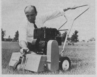
Ryan Equipment Co. has made available Ren-O-Thin, a new rental thatch-cutting and turf-renovating machine that limits user-adjustments to merely raising or lowering the cutting blades. The unit incorporates the design and construction of the institutional Ren-O-Thin but has eliminated the clutch and throttle for more maintenance-free operation in the rental market, says Ryan. Quick-change flail reels reduce costly down-time. For more details circle (706) on reply card.
