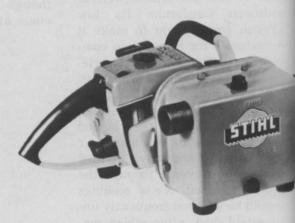
Stihl American, Inc., Midland Park, N. J., offers its 040 water pump with kit for replacing wearable parts. The  $1\frac{1}{2}$ -inch pump moves up to 4300 gallons per hour, with a total head of up to 160 feet. It offers self priming/cleaning action 'and is designed for long-life service, says Stihl. For more details circle (703) on reply card.
