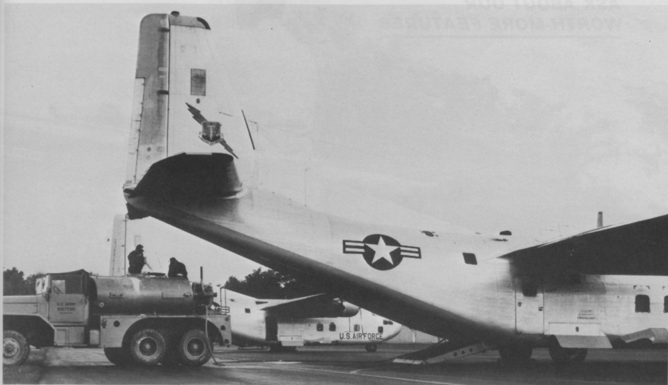
Sevin insecticide is pumped from army tank truck to waiting Air Force C-123 transport plane for spraying. Plane covers 500-foot swath.
