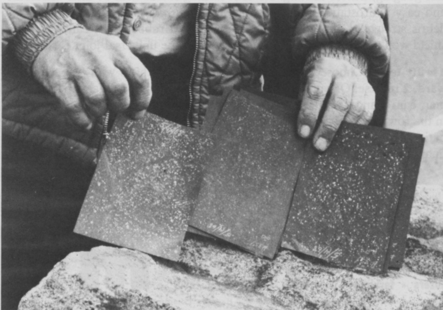
Cardboard check scraps help spraymen keep tab on effectiveness of insecticide coverage. Test here was made during spraying on New York's Bear Mountain.
