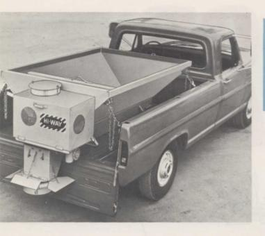
Self-contained, self-powered material spreader suitable for use on all light-duty trucks is announced by the HI-WAY Division of Highway Equipment Company, 616 "D" Ave., N.W., Cedar Rapids, lowa 52405. Utility unit converts any truck into a "spreader" on a moment's notice.
