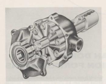
New 8-roller sprayer pump for high performance farm spraying has been announced by Hypro, Inc., 381 Fifth Avenue N.W., St. Paul, Minn. 55112. Special scoopless-rotor design reduces liquid by-pass problems and results in more liquid delivery at higher speeds and pressures. The pump, Series 7560C, delivers up to 18 gallons per minute, develops pressures up to 300 lbs. with 4½ horsepower, designed for direct drive by tractor power take-off. Can also be used with belt and pulley or gear head drive.
