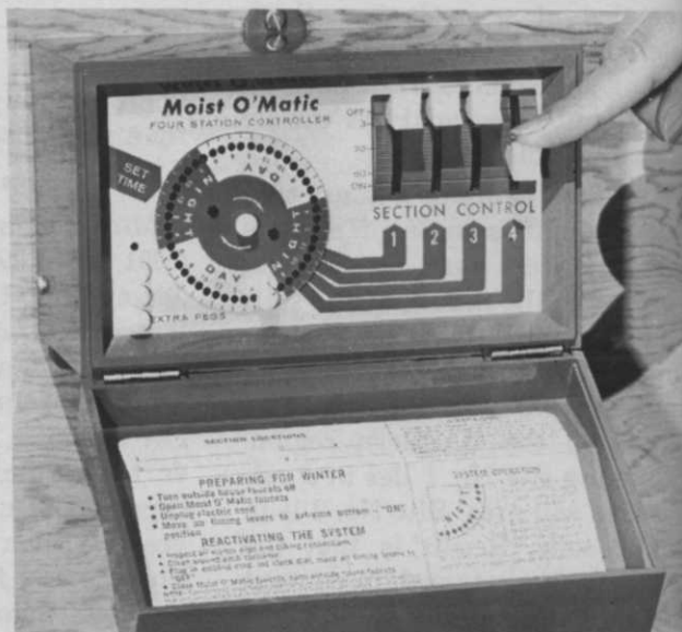
Compact Four Station Controller box regulates the system illustrated above.
