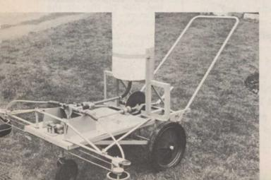
New sprayer featuring all fiberglass, non-corrosive tank, designed around a revolutionary sump-trap bottom is being manufactured by the Walsh Manufacturing Company, Box 351, Charles City, Ia. 50616. Tank has a 2-gallon sump trap outlet which completely empties each fill. Walsh "Posi-Sump" trap sprayer tanks are available in 110, 165, 200, 300 and 500 gallons capacity.
