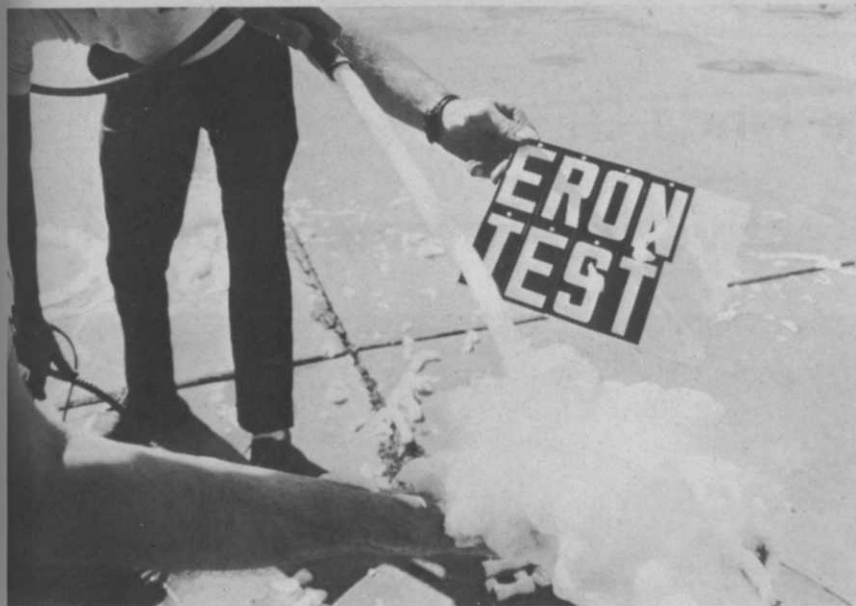
Eron foam generator will handle controlled volume of foamy herbicide in 12 mph wind according to the developer, Robert Eron. Unit can be used to spray minute amounts of foam on a single plant, or to deliver large quantities.
