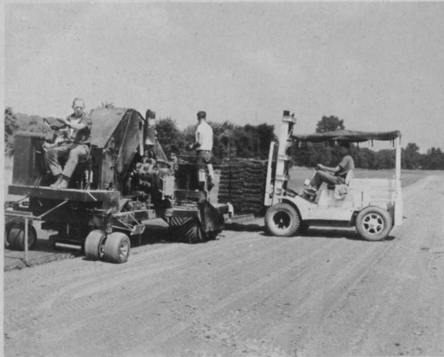
Fork lift, handled here by Charles Conrow, is used to pick up pallets behind harvest and load trucks for transport. The Rapps maintain two forklifts, one in the field and one which is towed behind a 10-wheel truck.
