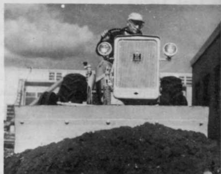
Front-mounted blade clears snow, grades crushed stone drives, dozes or spreads dirt. Features hydraulic control of height, manual angling of the blade to the right or left.
