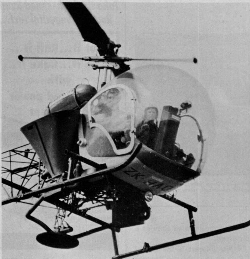
This Bell 47G-4 helicopter aids unsuccessful pine regeneration by distributing specially treated seeds over some 1500 acres of New Zealand forest-area.
