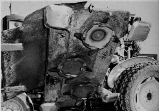
Rotary mower in tilted position showing mounting of the three 18-inch turbo cones.
