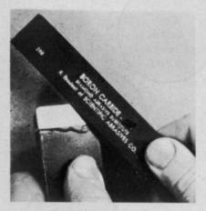
Boron Carbide Sharpeners that can replace steel files, honing stones and abrasive cloths are now available from Foster Enterprises, La Grange Park, III. Ideal for filing, edge finishing, dressing and polishing hardened tool steel, knives, bits, drills, and metal shears. Boron Carbide is tough, testing out next to diamond in hardness. It leaves a smooth, highly polished surface and removes scratches. Set of 3 (standard 1x8-in. size) consists of: 120 rough, 220 medium, 320 smooth. \$3.00 per set.
