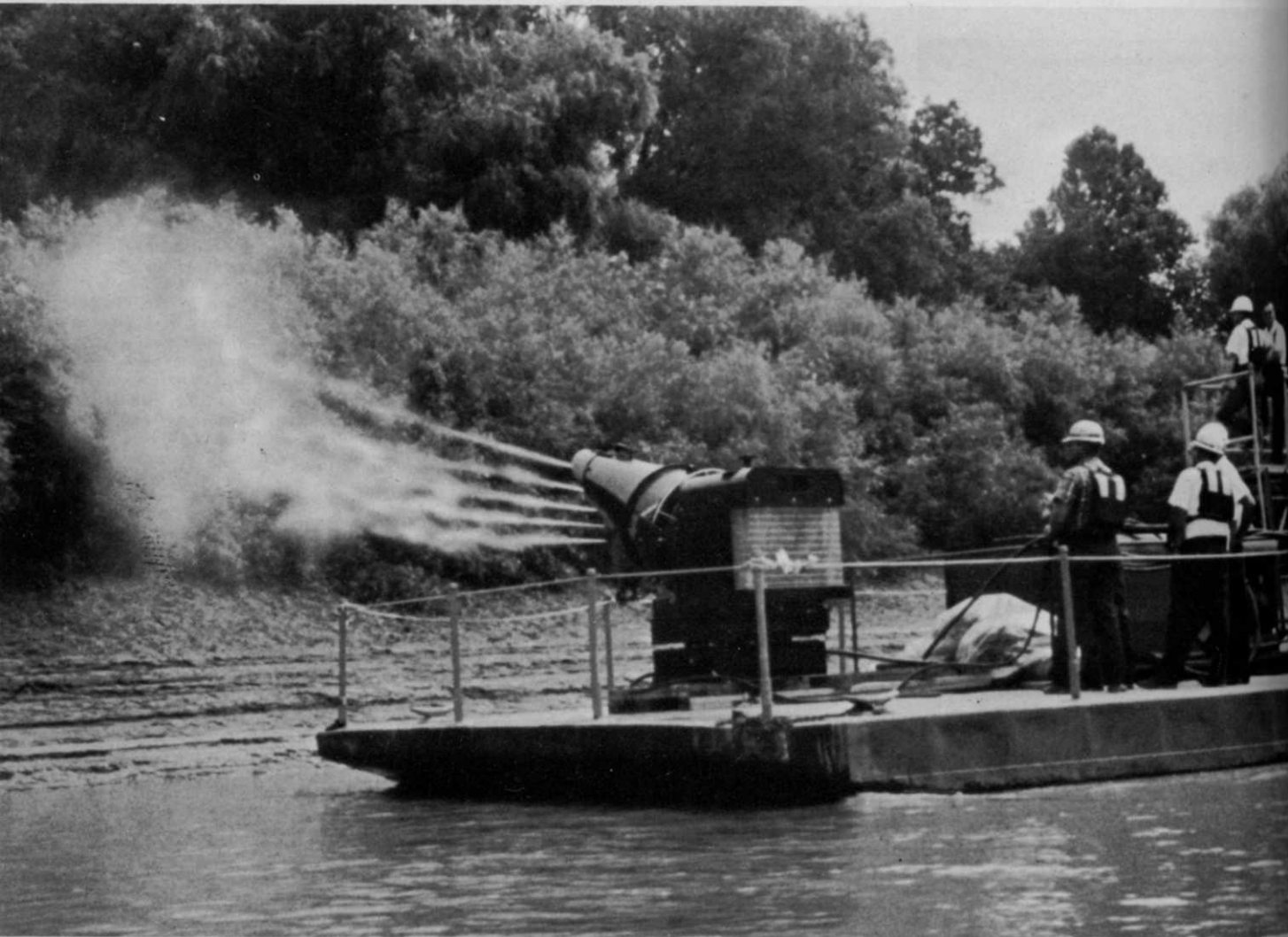
Spraying of vegetation along the Yazoo keeps fast-growing willows in check. Barge can spray 6 miles of riverbank daily.
