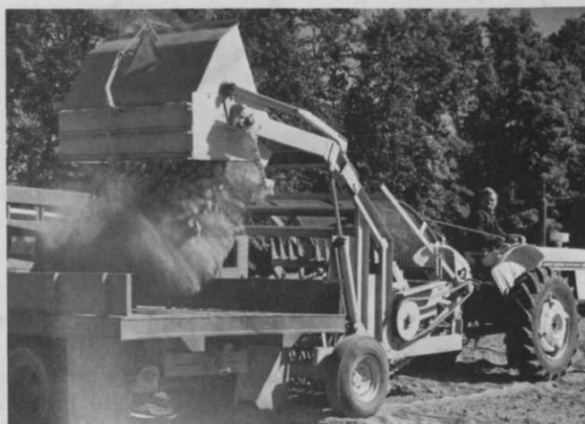
Stone picker is another important piece of equipment in the Smith mechanized operation. On large school landscaping job, cost of manual labor saved on this single job paid a big portion of first year's depreciation on the machine.
