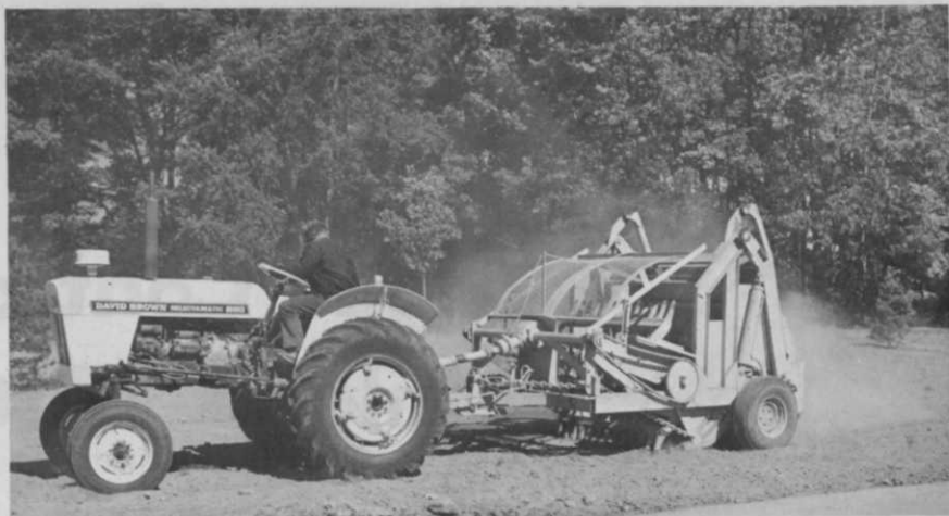
Stone picker is another important piece of equipment in the Smith mechanized operation. On large school landscaping job, cost of manual labor saved on this single job paid a big portion of first year's depreciation on the machine.
