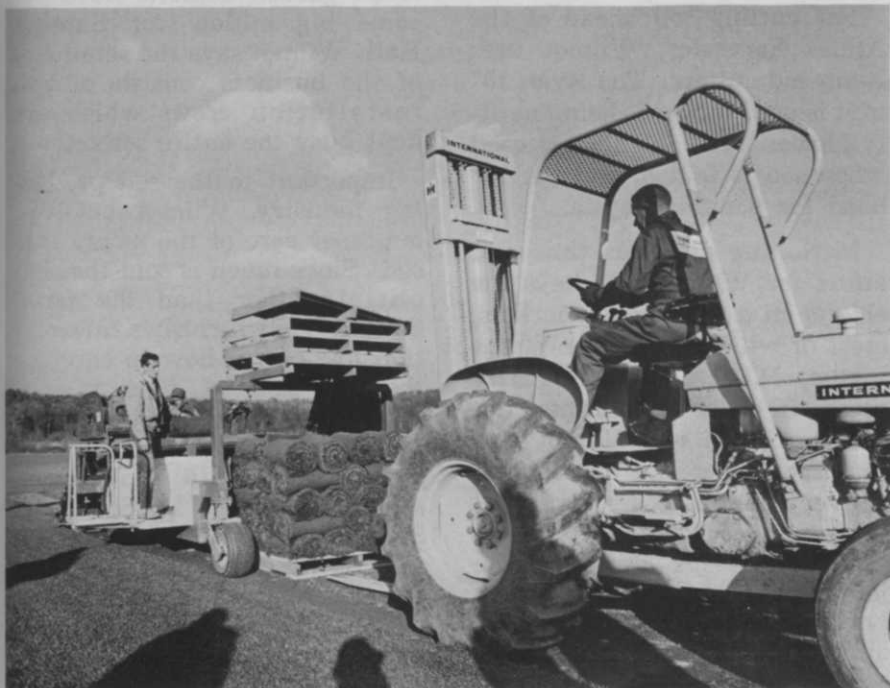
Fully mechanized system of sod harvesting on Summit Hall Turf Farm, Inc., is designed to prevent soil compaction. John Nunes sod harvester, above, and International Harvester forklift are on flotation tires. Forklift moves palletted sod to trucks located on hard surfaced roads.
