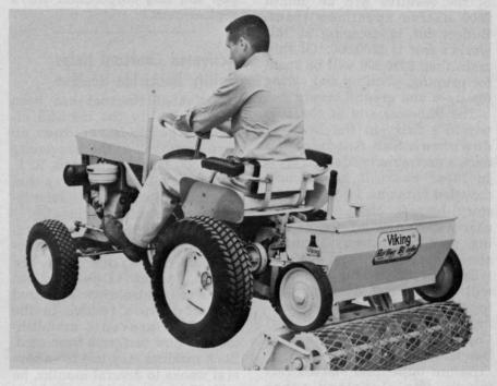
Kohler Co., Kohler, Wis., is introducing five vertical shaft engines for 1968. Model KV101 pictured, smallest of the five, is a compact, fourcycle, cast-iron engine which develops its rated 4 h.p. at 3600 rpm. Weight is 42 pounds, and measurements are  $12\frac{1}{2}$ " by  $12\frac{1}{6}$ " by  $10\frac{1}{4}$ " high. It is equipped with ACR, Kohler's patented automatic compression release for easy starting.
