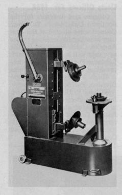
Fully-powered, air-electric Tire-Matic tire changer that handles tube-type as well as tubeless tires. Unit runs on 110 volt AC current, while bead breakers operate on 125 to 150 lbs. of air pressure. Write John Bean Automotive, FMC Corporation, 1305 S. Cedar St., Lansing, Mich. 48910.
