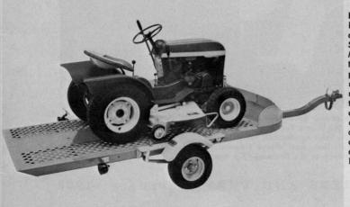
New tilt-deck utility trailer has been announced by the Snow Corp., 4350 McKinley, Omaha, Neb. 68112. Principal design improvements include a "loride" suspension system which decreases deck height; an increase in deck width; and a hydraulically controlled tilt mechanism on the three largest models.
