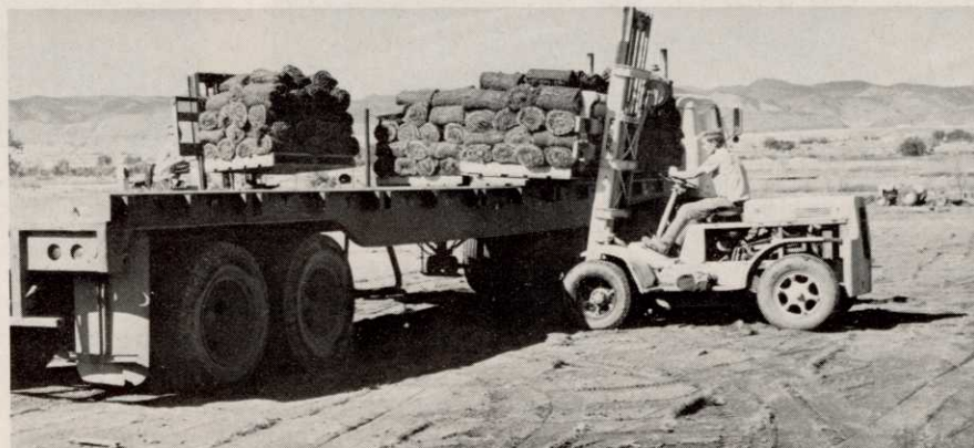
Once sod is palletted, fork lifts are used to quickly load trailer trucks. Loaded trucks are covered with a tarpaulin to protect sod from sun during transport. Tarp also helps hold sod rolls in place on pallets.
