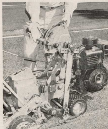
Specialty designed accessory helps maintain stability of cutting depth on cutter. Designed by Rusty Wilkins, it is transferred to new cutters as they are purchased.
