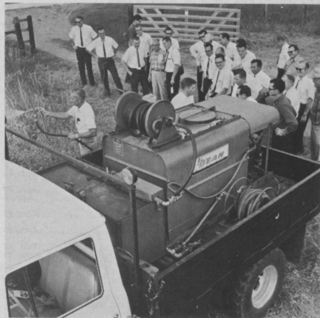
Ground spray rig with Stull bifluid system and John Bean equipment was used for weed and brush control demonstration.
