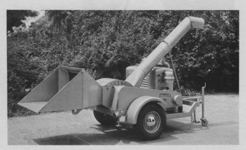
Mitts & Merrill, Inc., Saginaw, Mich., has made available 10 new Brush Chipper models that feature folding feed chutes for maneuvering ease and protection of cutting chamber. Staggered knife pattern on rotating cylinder provides smooth cutting action, shaves material into chips suitable for mulch. For more details circle (706) on reply card.
