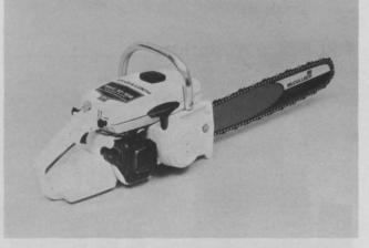
Los Angeles' McCulloch Corp. now offers MAC 10-10E, a self-contained electric starting chain saw. Batteries in handle supply starting power and are recharged automatically by alternator/generator while saw is on. 15-lb. unit offers fingertip chain oiling, noise muffler. For more details circle (705) on reply card.
