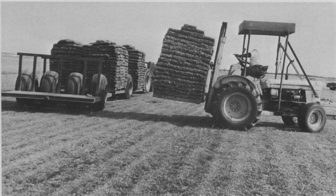
Like many progressive growers, Ousley has designed and built equipment to handle sod. This trailer unit equipped with airplane tires permits sod to be moved efficiently to heavy trucks on hard surfaced roads. The practice eliminates compaction in the field.
