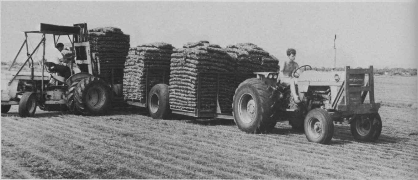
Forklifts are used in a pallet operation. All sod is folded and hand-loaded on pallets.
