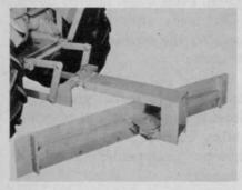
New attachment by Economy Tractor is rearmounted grader blade. As an aid to fine grading, landscaping, and other assignments, the blade can be angled in any of 5 positions. Write Engineering Products Co., 1005-HF Anoka Ave., Waukesha, Wis. 53186. (Circle No. 18 on Reader Card).
