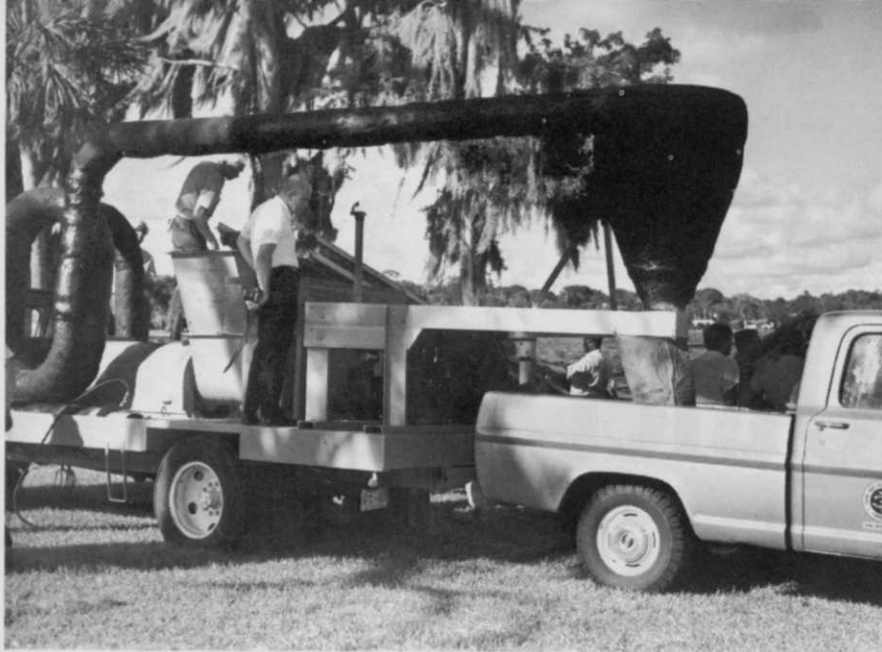
Many methods of handling residue of harvested aquatic weeds have been tried. Among new innovations under trial is this new piece of equipment, designed for pelletizing to be used as cattle feed.
