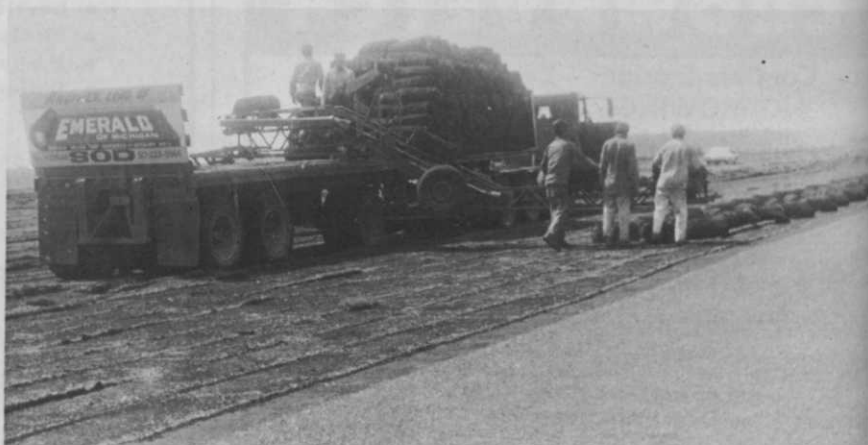
Daymon uses 18-wheel drive truck tractor with side loading conveyor for trailer in moving harvested sod from field.
