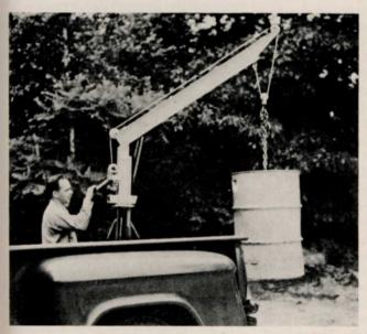
Weldex is marketing new utility truck crane. Lifting is done by a lug-All cable winch-hoist instead of the usual hydraulic cylinder or jack. Produces high lifting capacity, positive and accurate lowering of the load, no pulling-in of load being lifted. Winch-hoist detaches from the crane and can be used as standard come-a-long. Boom rotates 360°. Crane bolts to any size truck. Information from Weldex, Old Westboro Road, Grafton, Mass. 01519.
